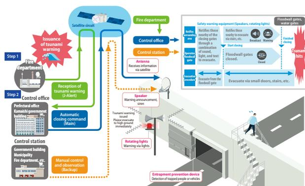
Automatic closing system mechanism
