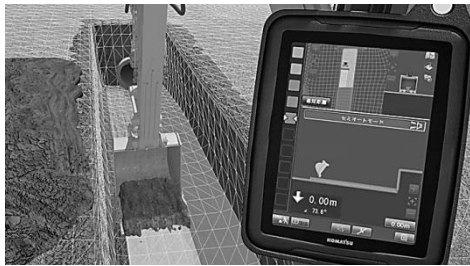
(ICT 建機の操縦室画面)
